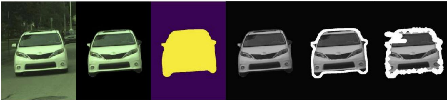
Figure 10: Input data preparation for training the synthesis network. From left to right: scene image I , object segment S and mask M and three random data augmentation including color-jitter, segment boundaries erosion-expansion and random mask in the boundary.
