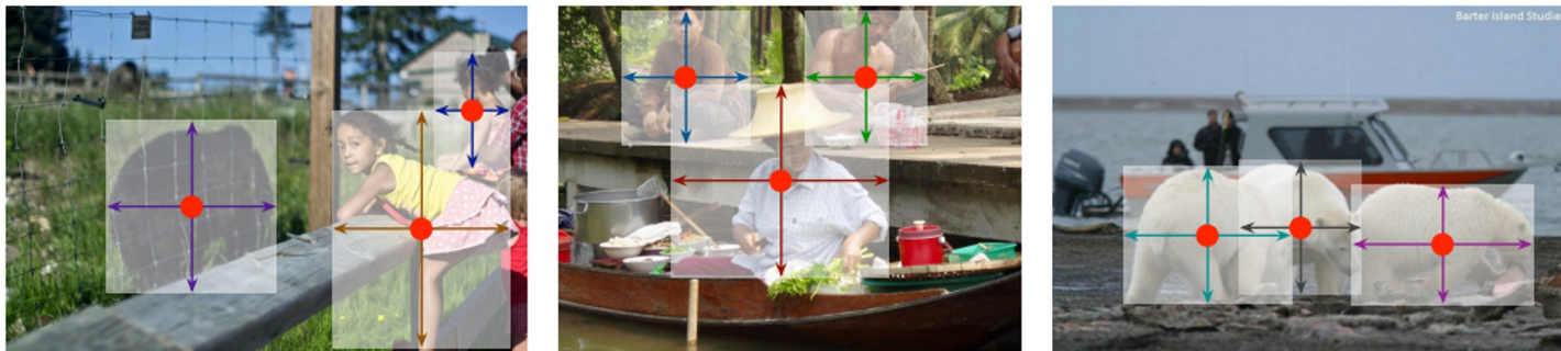
Figure 2: We model an object as the center point of its bounding box. The bounding box size and other object properties are inferred from the keypoint feature at the center. Best viewed in color.
